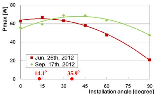
Fig. 5 Pmax when installation angle changes (experiments in June and September)
