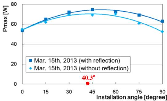
Fig. 9 Pmax when installation angle changes (examination of sunlight reflection)
