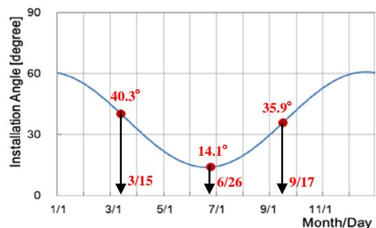
Fig. 6 Optimum installation angle (theoretical data and date of experiments)
