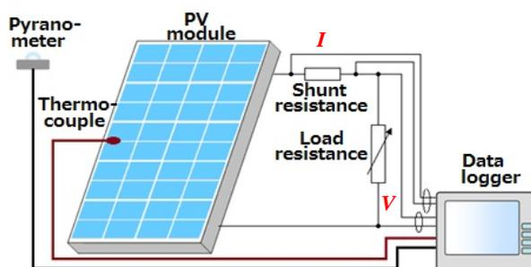
Fig. 3 Measurement system for PV module
