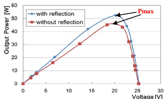
Fig. 8  $P$ - $V$  characteristics (examination of sunlight reflection)
