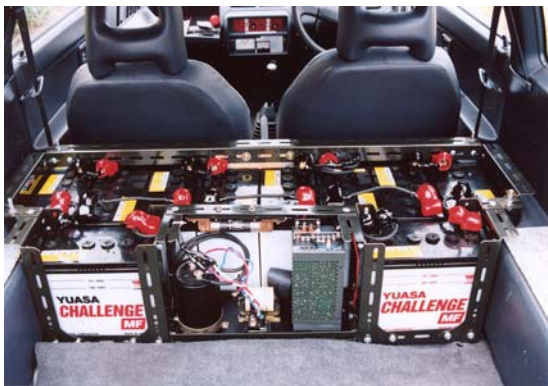
Fig. 3 Battery arrangement (NEV-I)
